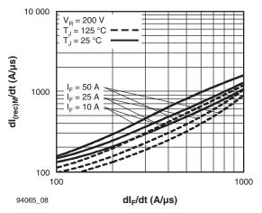
Fig. 8 - Typical  $dI_{(rec)M}/dt$  vs.  $dI_F/dt$
