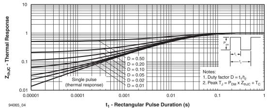
Fig. 4 - Maximum Thermal Impedance Z<sub>th,IC</sub> Characteristics
