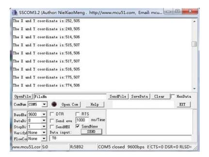
The output value from the analog port of Arduino can be converted to the corresponding resistance by using the formula:R=(float)(1023-sensorValue)\*10/sensorValue.
