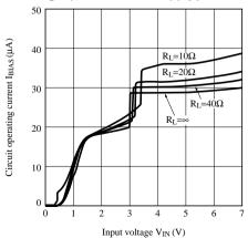
Fig.4 Overcurrent Protection Characteristics (Typical Value)
