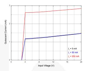
Figure 10. Quiescent Current vs. Input Voltage
