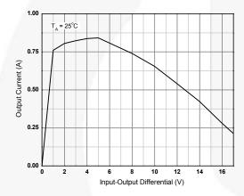
Figure 5. Peak Output Current
