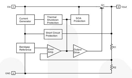
Figure 1. Block Diagram
