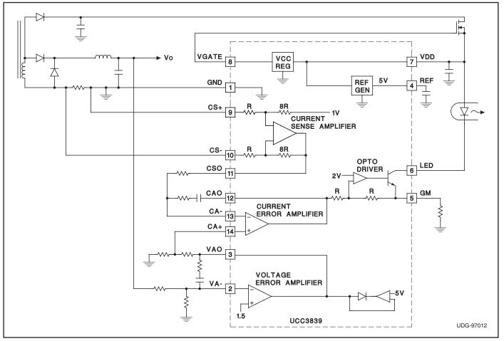
Figure 1. Secondary side average current mode controller.
