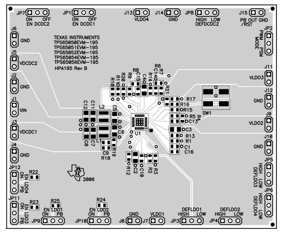
Figure 1. Assembly Layer
