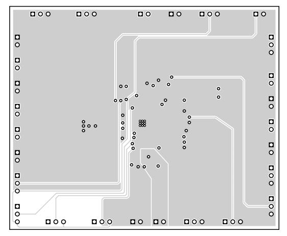
Figure 3. Inner Layer 2 Routing
