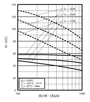
Fig. 5 - Typical Reverse Recovery Time vs. dl<sub>F</sub>/dt
