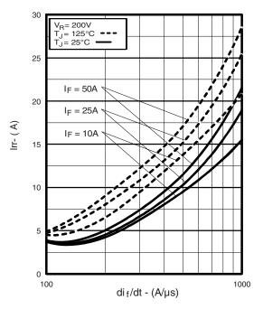
Fig. 6 - Typical Recovery Current vs.  $dI_{\mbox{\scriptsize F}}/dt$
