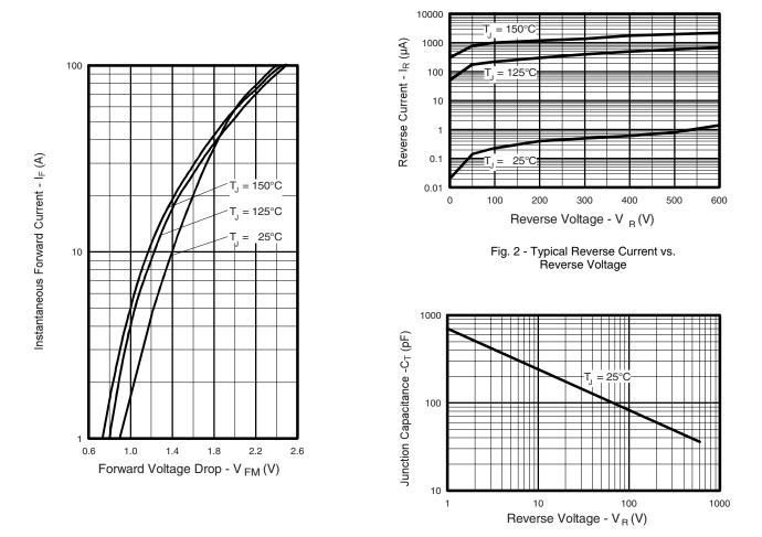
Fig. 1 - Maximum Forward Voltage Drop vs. Instantaneous Forward Current
