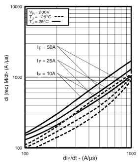
Fig. 8 - Typical  $dI_{(rec)M}/dt vs. dI_F/dt$
