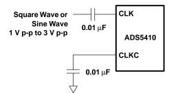
Figure 26. AC-Coupled Single-Ended Clock Input
