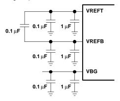
Figure 25. Internal Reference Usage
