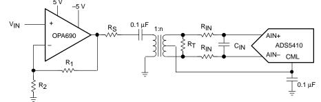
Figure 23. Converting a Single-Ended Input Signal Into a Differential Signal Using an RF Transformer
