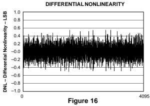
150% duty cycle. AV<sub>DD</sub> = 3.3 V, DV<sub>DD</sub> = 1.8 V, DV<sub>DD</sub> = 1.8 V
