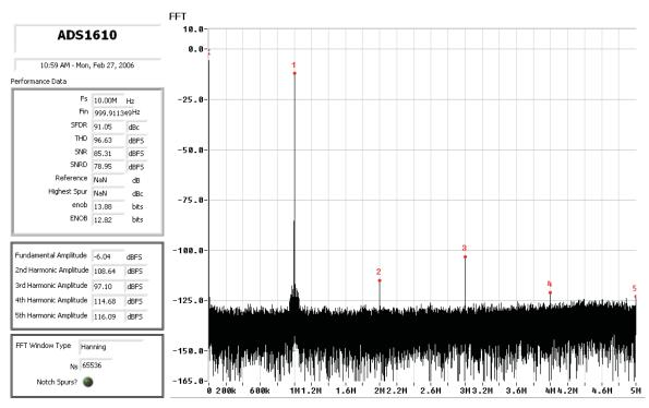
Figure 7. Test Results With a 1-MHz Input
