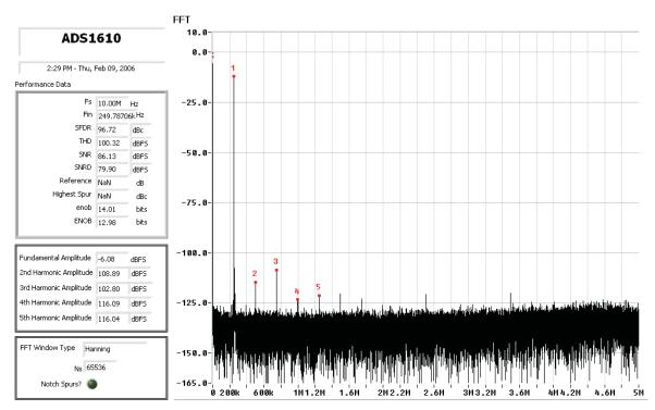
Figure 5. Test Results With a 250-kHz Input
