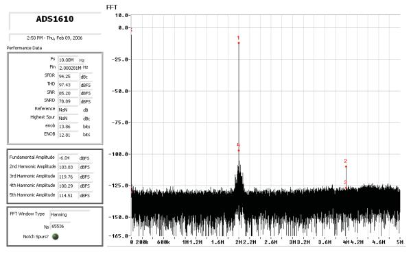
Figure 8. Test Results With a 2-MHz Input
