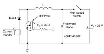
Fig. 8 - Unclamped Inductive Test Circuit
