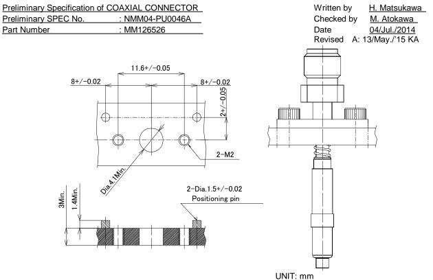
Figure.5 Machine's hole diameter for attachment probe
