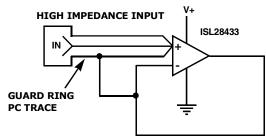
FIGURE 43. USE OF GUARD RINGS TO REDUCE
