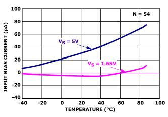
FIGURE 4. MEDIAN  $I_{B+}$  vs TEMPERATURE
