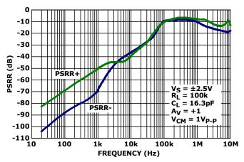
FIGURE 23. PSRR vs FREQUENCY,  $V_S = \pm 2.5V$
