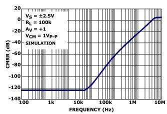
FIGURE 22. CMRR vs FREQUENCY,  $V_S = \pm 2.5V$
