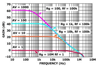
FIGURE 50. SIMULATED FREQUENCY RESPONSE vs **CLOSED LOOP GAIN**
