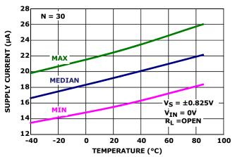
FIGURE 8. SUPPLY CURRENT vs TEMPERATURE
