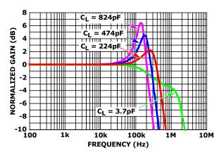
FIGURE 52. SIMULATED GAIN vs FREQUENCY vs CL
