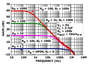
FIGURE 49. CHARACTERIZED FREQUENCY RESPONSE **vs CLOSED LOOP GAIN**
