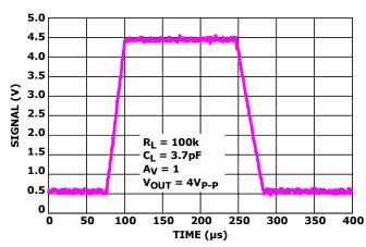
FIGURE 27. LARGE SIGNAL STEP RESPONSE (4V)
