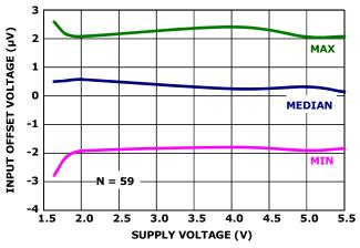
FIGURE 1. INPUT OFFSET VOLTAGE vs SUPPLY VOLTAGE
