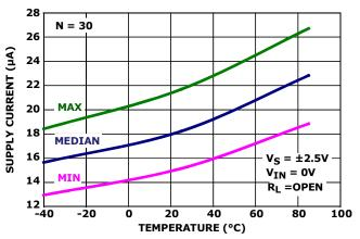
FIGURE 9. SUPPLY CURRENT vs TEMPERATURE
