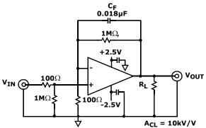
FIGURE 44. HIGH GAIN, PRECISION DC-COUPLED **AMPLIFIER**
