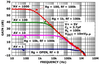
FIGURE 19. FREQUENCY RESPONSE vs CLOSED LOOP
