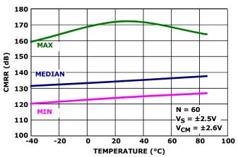
FIGURE 25. CMRR vs TEMPERATURE
