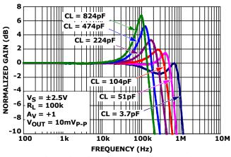
FIGURE 21. GAIN vs FREQUENCY vs C<sub>1</sub>
