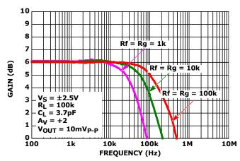
FIGURE 17. GAIN vs FREQUENCY vs FEEDBACK RESISTOR VALUES  $R_f/R_\alpha$
