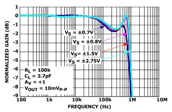
FIGURE 20. GAIN vs FREQUENCY vs SUPPLY VOLTAGE
