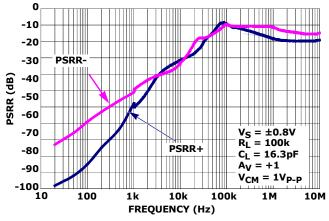
FIGURE 24. PSRR vs FREQUENCY,  $V_S = \pm 0.8V$
