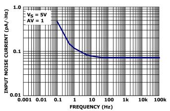
FIGURE 12. INPUT NOISE CURRENT DENSITY vs FREQUENCY
