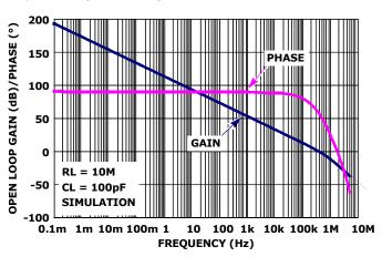
FIGURE 14. FREQUENCY RESPONSE vs OPEN LOOP GAIN,  $R_L = 10 M\Omega$
