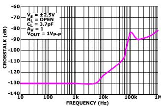
FIGURE 33. CROSSTALK vs FREQUENCY,  $V_S = \pm 2.5V$
