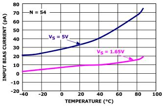
FIGURE 5. MEDIAN  $I_{B-}$  vs TEMPERATURE
