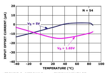
FIGURE 6. MEDIAN  $I_{\mbox{OS}}$  vs SUPPLY VOLTAGE vs TEMPERATURE
