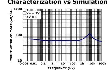
FIGURE 47. CHARACTERIZED INPUT NOISE VOLTAGE **DENSITY vs FREQUENCY**
