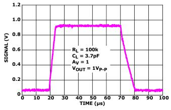
FIGURE 28. LARGE SIGNAL STEP RESPONSE (1V)
