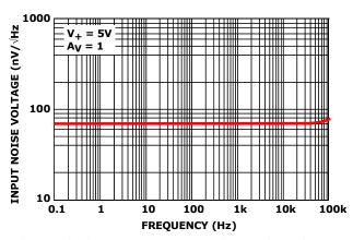
FIGURE 48. SIMULATED INPUT NOISE VOLTAGE **DENSITY vs FREQUENCY**
