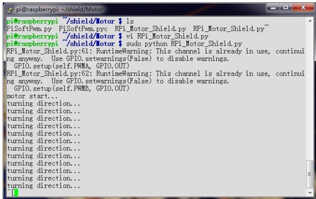
The screenshot shows a terminal window titled "pi@raspberrypi: ~/shield/Motor". The user runs "ls" to list files, then "vi RPi\_Motor\_Shield.py" to edit the script. Finally, they run "sudo python RPi\_Motor\_Shield.py". The output shows the script starting a motor and then printing "turning direction..." repeatedly, indicating alternating forward and backward motion. There are several runtime warnings about GPIO channels being already in use.
