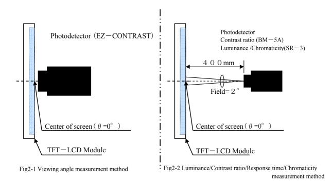
Fig2 Optical characteristics measurement method
