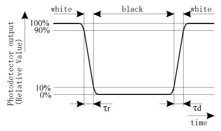
[Note9-4] This parameter should be measured at the center of the screen and 30 minutes after turn-on.
