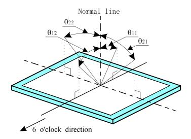
The best viewing angle of this module is slightly leaned to 6 o'clock from normal line.
