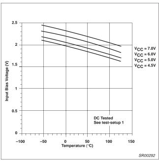
Figure 20. Input Bias Voltage vs Temperature
