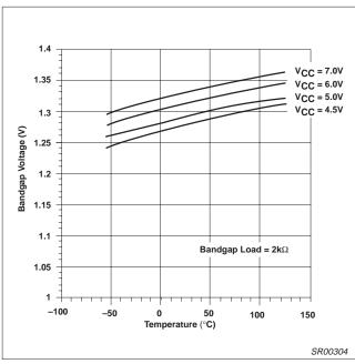
Figure 32. Bandgap Voltage vs Temperature and  $V_{CC}$
