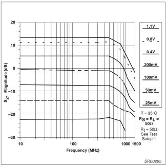
Figure 23. Insertion Gain vs Frequency and V<sub>AGC</sub>
