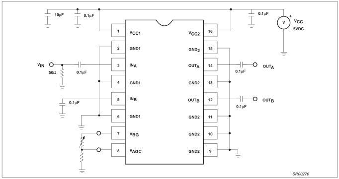
Figure 4. VGA AC Evaluation Board
