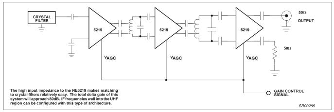
Figure 13. Receiver AGC IF Gain
