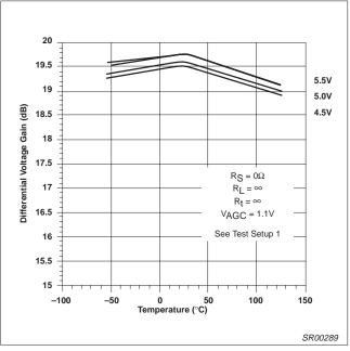
Figure 17. Voltage Gain vs Temperature and  $V_{\mbox{\footnotesize CC}}$
