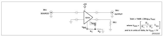
Figure 11. User-Programmable Fixed Gain Block
