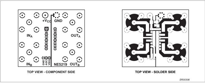
Figure 34. VGA AC Evaluation Board Layout (DIP Package)
