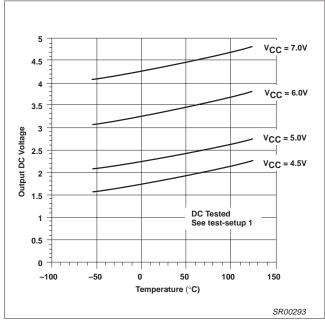
Figure 21. Output Bias Voltage vs Temperature and  $\rm V_{\rm CC}$
