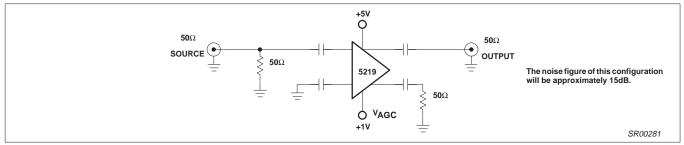
Figure 9. Simple Amplifier Configuration
