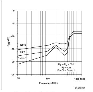
Figure 26. Output Return Loss vs Frequency
