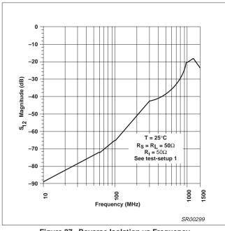
Figure 27. Reverse Isolation vs Frequency
