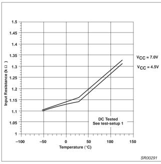
Figure 19. Input Resistance vs Temperature
