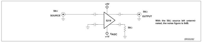
Figure 10. Unterminated Configuration
