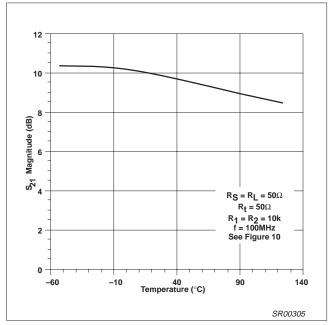
Figure 33. Fixed Gain vs Temperature
