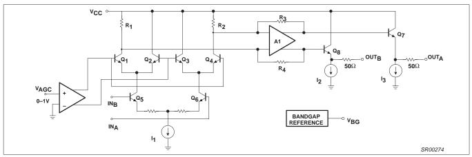
Figure 2. Equivalent Schematic of VGA
