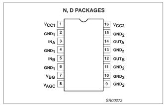
Figure 1. Pin Configuration
