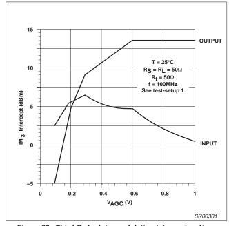
Figure 29. Third-Order Intermodulation Intercept vs  $V_{\mbox{\scriptsize AGC}}$
