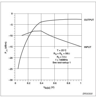
Figure 28. 1dB Gain Compression vs V<sub>AGC</sub>
