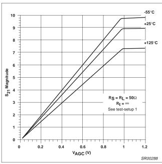
Figure 16. Insertion Gain vs  $V_{\mbox{\scriptsize AGC}}$  and Temperature
