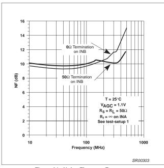
Figure 31. Noise Figure vs Frequency
