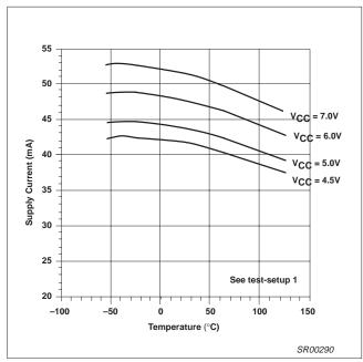
Figure 18. Supply Current vs Temperature and  $V_{\text{CC}}$
