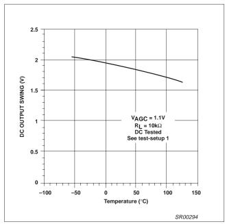
Figure 22. DC Output Swing vs Temperature
