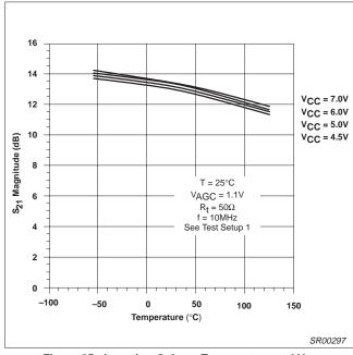
Figure 25. Insertion Gain vs Temperature and  $V_{\text{CC}}$
