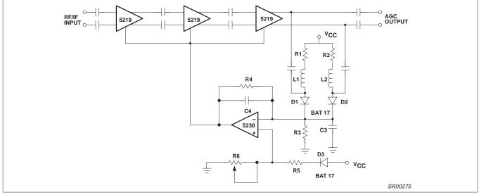
Figure 3. AGC Configuration Using Cascaded SA5219s
