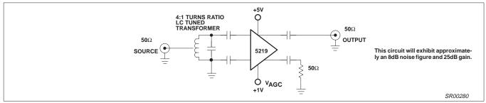
Figure 8. Narrowband Gain Optimization
