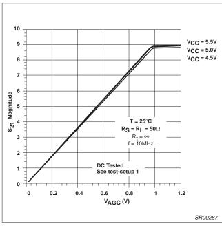
Figure 15. Gain vs V<sub>AGC</sub> and V<sub>CC</sub>
