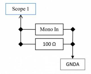
Mono Connection-Mono/Stereo Connector
