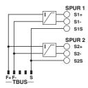
Figure 2 FB-2SP/24DC circuit diagram
