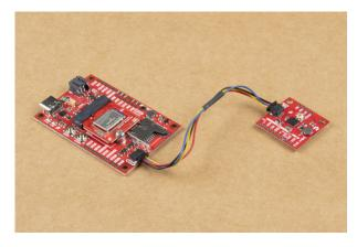
Before powering everything up, insert your microSD card into the card slot and press it in to lock it into place.
