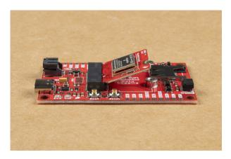
Once the board is in the socket, gently press the Processor Board down, grab the set screw and tighten it with a Phillip's head screwdriver:
