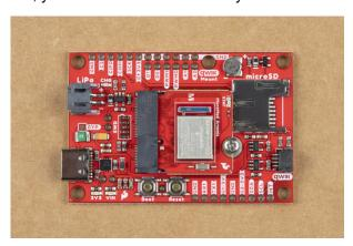
**Note:** There is *technically* no way to insert the processor backward since the key prevents it from mating with the M.2 connector. As an extra safeguard to prevent inserting a processor improperly or with a poor connection, the mounting screw will not match up if the Processor Board is not plugged in entirely.
