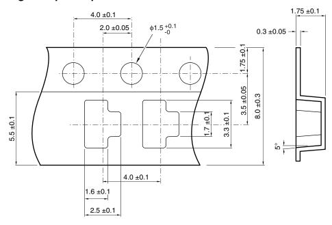
Fig. 6 Reel Shape and Dimension
