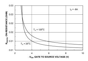
Figure 4. On-Resistance Variation with Gate-to-Source Voltage.
