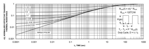
Figure 11. Transient Thermal Response Curve.
