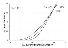
Figure 5. Transfer Characteristics.
