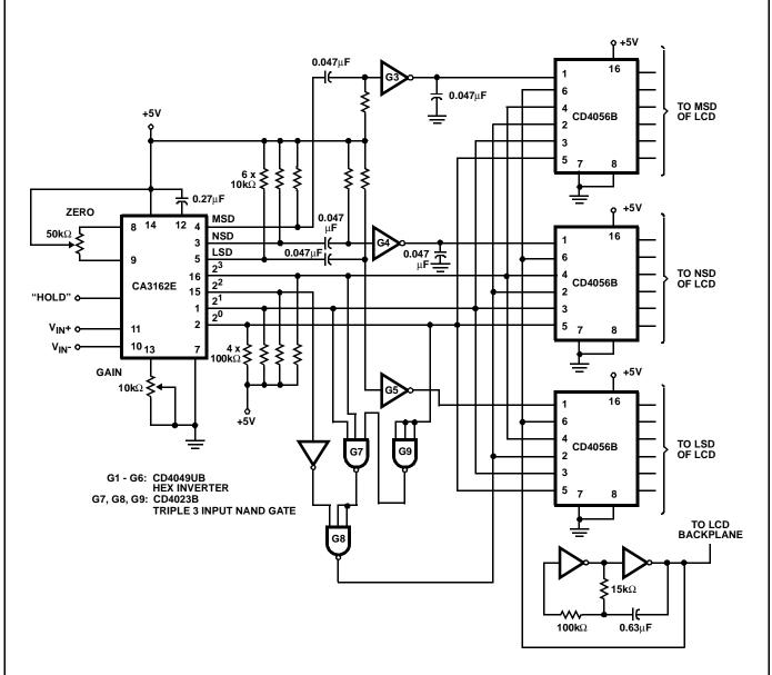
FIGURE 3. TYPICAL LCD APPLICATION
