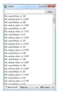
As default, Vref is generated by Arduino which is theoretically 5V. But actually that is a value afloat which results the deviation of the final data. This kind of inaccuracy is avoided when using Grove - I2C ADC, because it provides a strict 3.0V as Vref. To contrast, in the same condition, sensor values collected by the circuit with Grove - I2C ADC in the scope is shown below:
