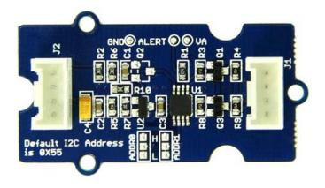
Grove - I2C ADC is a 12-bit precision ADC module based on ADC121C021. It helps you increase the accuracy of value collected from analog sensor by providing a constant reference voltage. Because its address is changeable, you can use up to 9 I2C ADC at the same time at most. At the other hand, this module provides auto sleep function which lowers the power consumption considerably.
