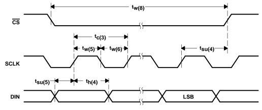
Figure 2–4. Three-Wire Control Interface Timing Requirements
