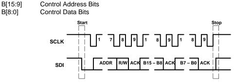
Figure 3–2. 2-Wire Compatible Timing
