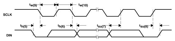
Figure 2–5. Two-Wire Control Interface Timing Requirements
