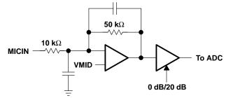
Figure 3–4. Microphone Input Circuit
