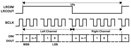
Figure 3–6. Left-Justified Mode Timing
