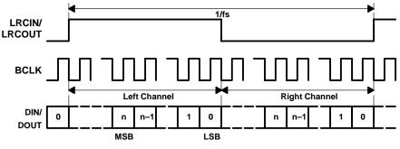
Figure 3–5. Right-Justified Mode Timing
