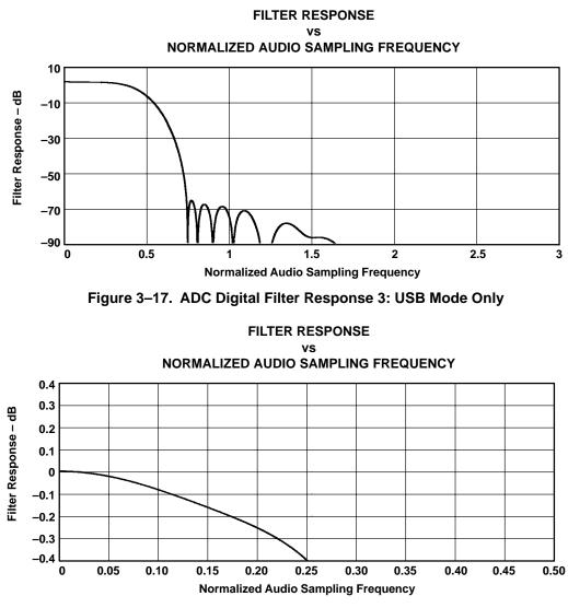
Figure 3–18. ADC Digital Filter Ripple 3: USB Mode Only
