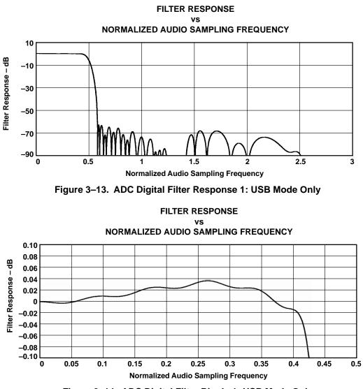
Figure 3–14. ADC Digital Filter Ripple 1: USB Mode Only
