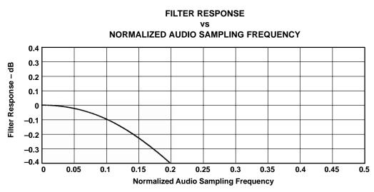
Figure 3–16. ADC Digital Filter Ripple 2: USB Mode and Normal Modes
