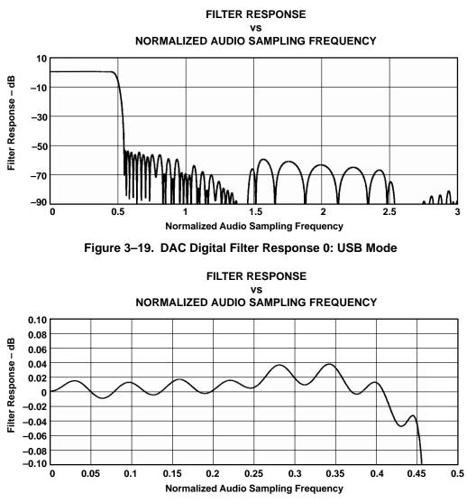
Figure 3–20. DAC Digital Filter Ripple 0: USB Mode
