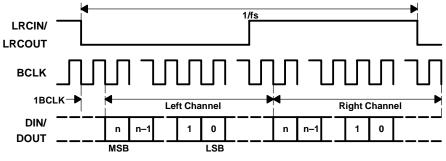
Figure 3–7. I<sup>2</sup>S Mode Timing
