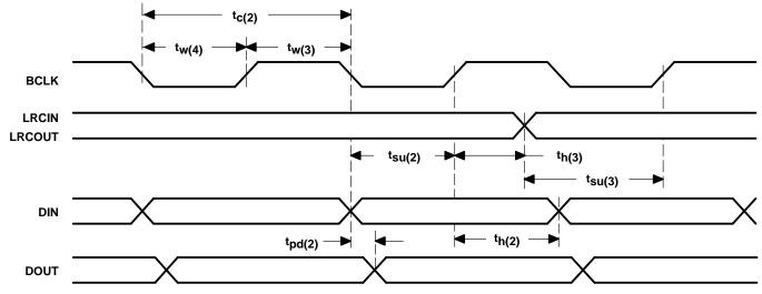
Figure 2–3. Slave-Mode Timing Requirements
