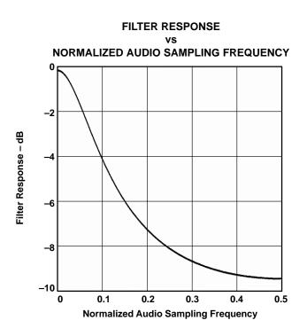
Figure 3–9. Digital De-Emphasis Filter Response – 44.1 kHz Sampling
