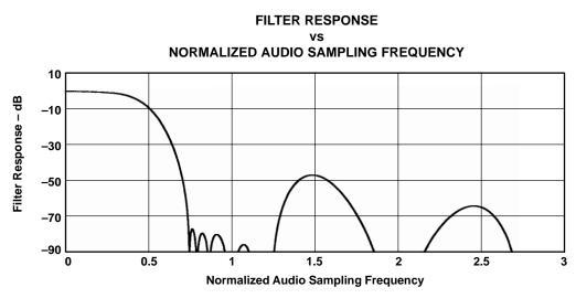
Figure 3–15. ADC Digital Filter Response 2: USB mode and Normal Modes (Group Delay = 3 Output Samples)
