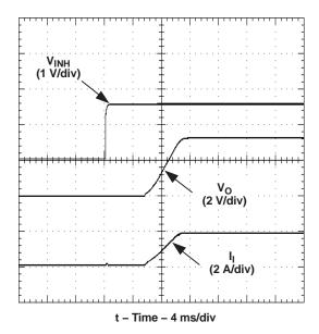
Figure 15. Power Up Response From Inhibit Control
