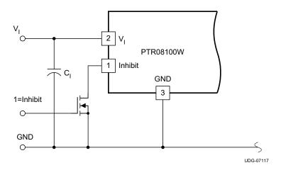
Figure 14. On/Off Inhibit Control Circuit
