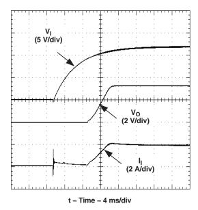
Figure 13. Power-Up Waveforms
