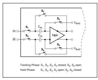
FIGURE 1. Simplified Circuit of Input Track-and-Hold Amplifier of ADS5220.
