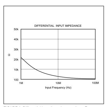
FIGURE 2. Differential Input Impedance vs Input Frequency.
