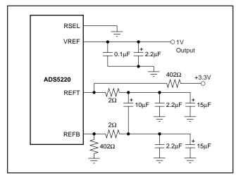
FIGURE 7. Internal Reference Mode for  $V_{RFF} = 1V$ .
