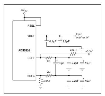
FIGURE 10. External Reference Configuration.
