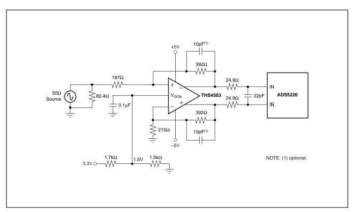
FIGURE 4. Using the THS4503 Differential Amplifier (Gain = 2) to Drive the ADS5220 in a DC-Coupled Configuration.
