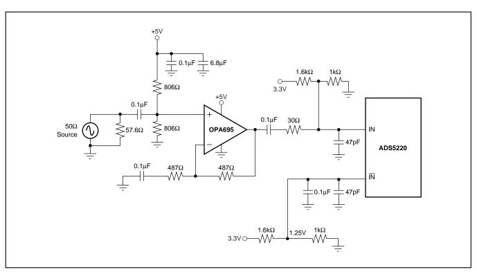
FIGURE 5. Single-Ended Input of ADS5220 Driven by OPA695 with Gain = 2.
