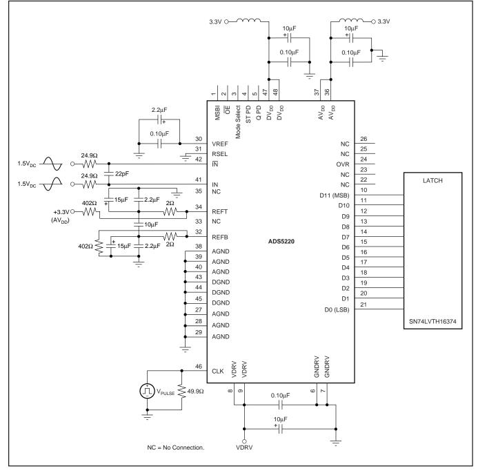
FIGURE 11. General Configuration for the ADS5220.
