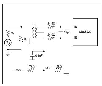
FIGURE 3. Transformer-Coupled Differential Input Configuration of ADS5220.
