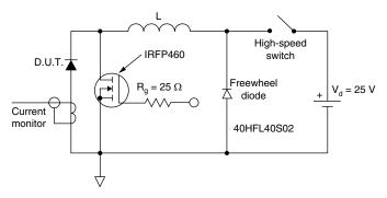
Fig. 8 - Unclamped Inductive Test Circuit
