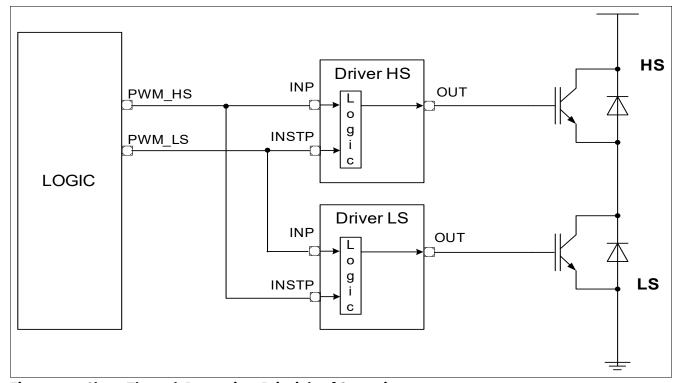
Figure 24 Shoot Through Protection: Principle of Operation
