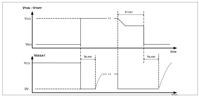
Figure 20 DESAT Operation
