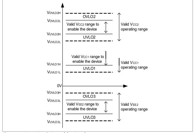
Figure 23 Power Supply Supervision Function
