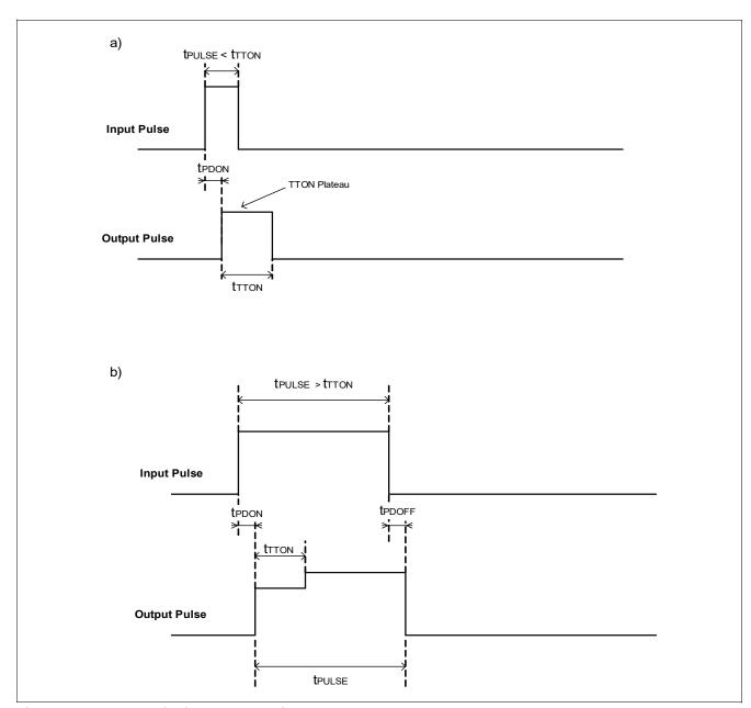
Figure 14 TTON: Principle of Operation
