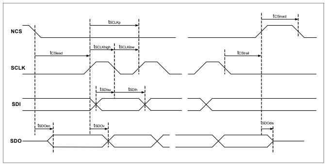
Figure 29 SPI Interface Timing
