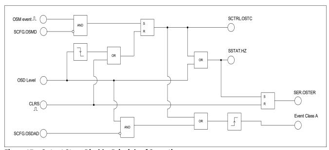
Figure 17 Output Stage Disable: Principle of Operation
