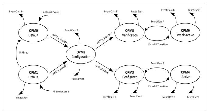
Figure 11 Operating Modes State Diagram
