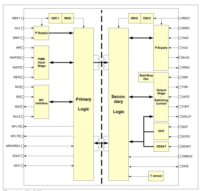
Figure 2 Block Diagram
