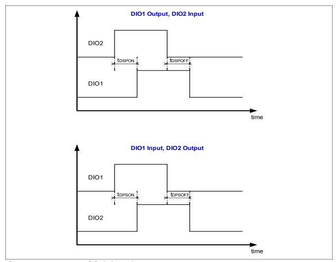
Figure 18 Low Latency Digital Channel
