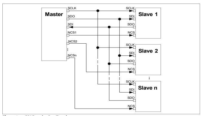
Figure 6 SPI Regular Bus Topology
