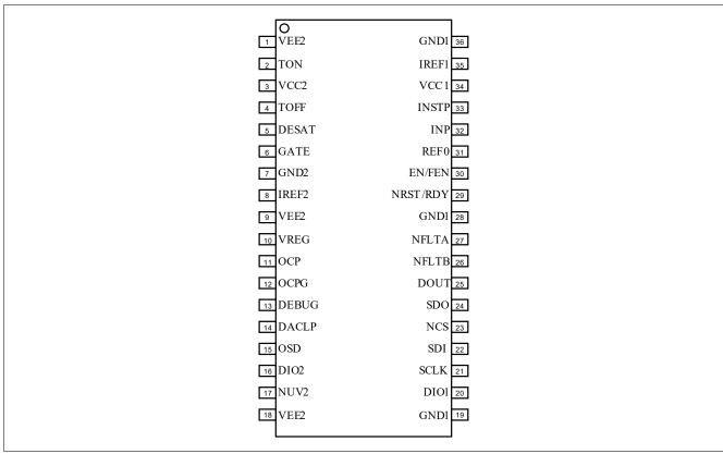
Figure 1 **Pin Configuration**
