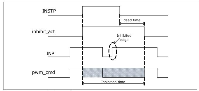
Figure 5 STP: Example of Operation
