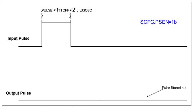
Figure 15 TTOFF: pulse suppressor aborting a turn-on sequence
