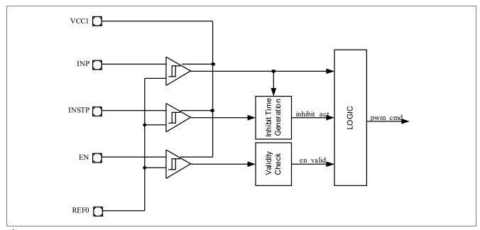
Figure 3 PWM Input Stage
