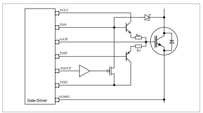
Figure 12 Output Stage Diagram of Principle
