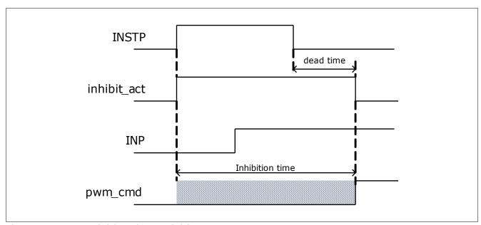
Figure 4 STP: Inhibition Time Definition
