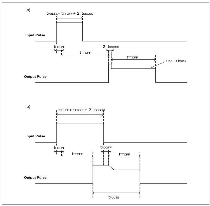
Figure 13 TTOFF: Principle of Operation
