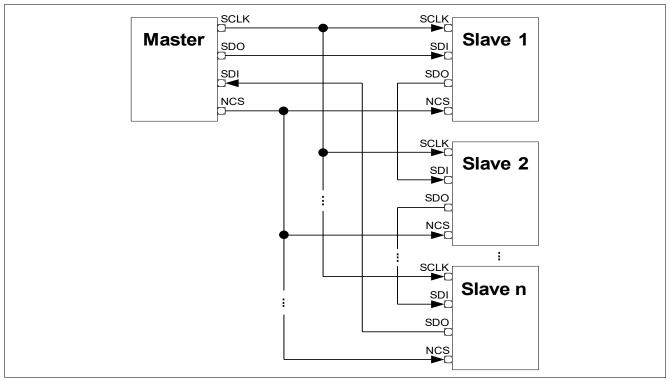
Figure 7 SPI Daisy Chain Bus Topology
