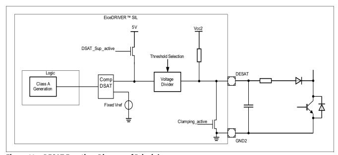
Figure 19 DESAT Function: Diagram of Principle
