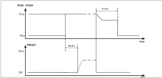
Figure 21 DESAT Operation with DESAT clamping enabled
