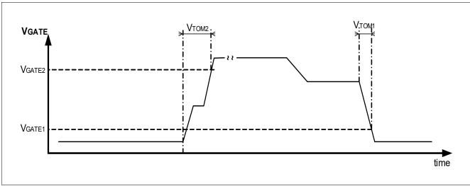
Figure 25 Gate Monitoring Function: Timing Definition
