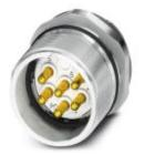
Device connector for front wall, straight, shielded: yes, SPEEDCON locking, M23, Number of positions: 8+1, Type of contact: Male connector, Solder connection, Seal, axial, Central fastening Pg13,5
