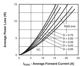
Fig. 6 - Forward Power Loss Characteristics
