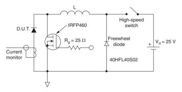
Fig. 8 - Unclamped Inductive Test Circuit
