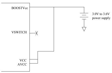
Figure 4-3. Power Supply Connection Without Booster
