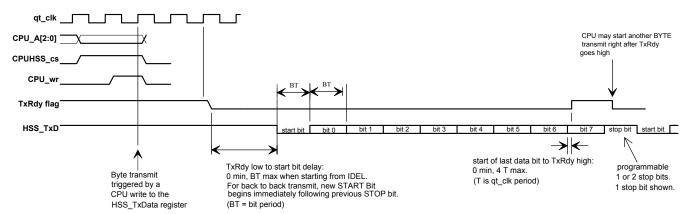
qt\_clk, CPU\_A, CPUHSS\_cs, CPU\_wr are internal signals, included in the diagram to illustrate relationship between CPU operations and HSS port operations.
