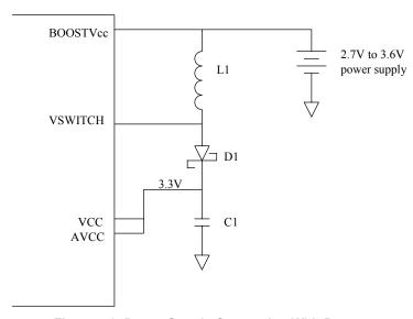
Figure 4-2. Power Supply Connection With Booster
