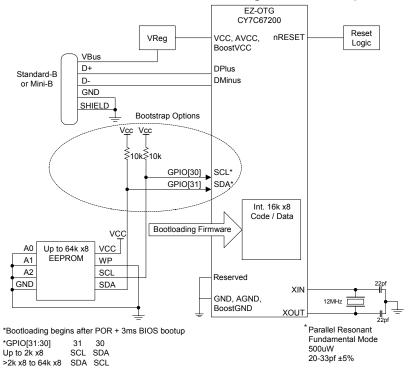
Figure 4-5. Minimum Standalone Hardware Configuration – Peripheral Only
