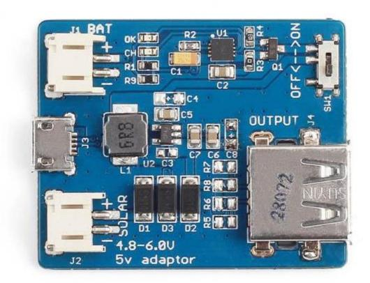
Power your favourite electronic kit with green energy! The Lipo Rider board allows you ride the solar wave to run your favourite 5V device. The Lipo Rider board is the ideal green power solution for your outdoor sensor design. Attach the Lipo Rider board to your sensor board and it can run on solar power forever!
