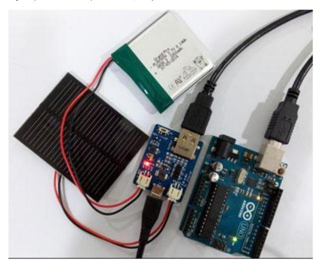
Lipo Rider powering an Arduino Duemilanove (not strictly an outdoor sensor in this case as I have not connected any sensor and it is not outdoor, but you get the point )
