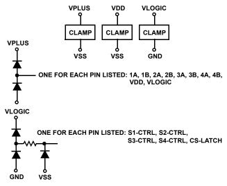
FIGURE 7. ESD/OVERVOLTAGE PROTECTION
