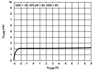
FIGURE 25. OFF-LEAKAGE vs SWITCH VOLTAGE
