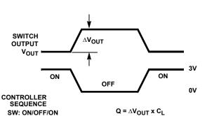
Switch changes state on rising edge of CS-LATCH.
