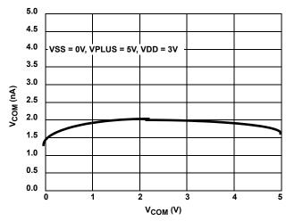
FIGURE 16. ON-LEAKAGE vs SWITCH VOLTAGE
