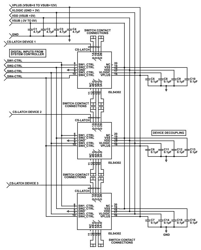
FIGURE 8. ISL54302 SW-CONTROL LINES MULTIPLEXED
