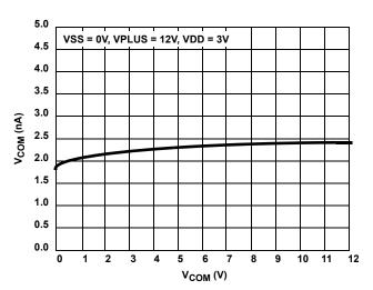
FIGURE 20. ON-LEAKAGE vs SWITCH VOLTAGE
