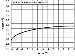
FIGURE 19. ON-LEAKAGE vs SWITCH VOLTAGE
