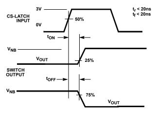
Switch changes state on rising edge of CS-LATCH.  $V_{NA}$  = VOUT at all times.
