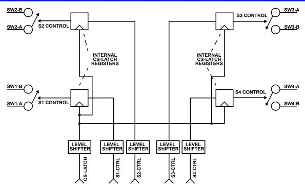
FIGURE 6. ISL54302 FUNCTIONAL DIAGRAM
