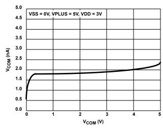
FIGURE 22. OFF-LEAKAGE vs SWITCH VOLTAGE
