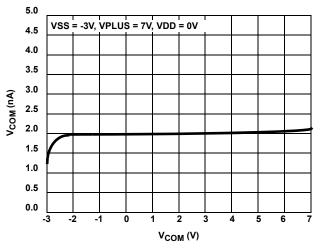
FIGURE 17. ON-LEAKAGE vs SWITCH VOLTAGE
