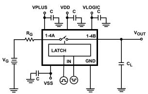
Repeat test for all switches.  $C_L$  includes fixture and stray capacitance.
