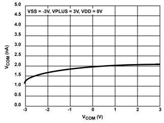
FIGURE 15. ON-LEAKAGE vs SWITCH VOLTAGE
