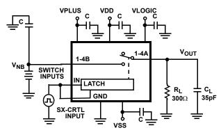
Repeat test for all switches. C<sub>L</sub> includes fixture and stray capacitance.
