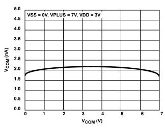
FIGURE 18. ON-LEAKAGE vs SWITCH VOLTAGE
