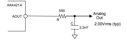
(fc = 129kHz, gain = -0.4dB @ 40kHz, gain = -1.4dB @ 80kHz)
