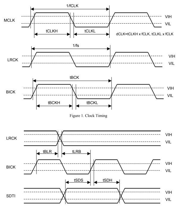
Figure 2. Serial Interface Timing
