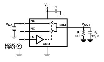
C<sub>L</sub> includes fixture and stray capacitance.
