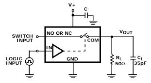
Repeat test for all switches. C<sub>L</sub> includes fixture and stray capacitance.
