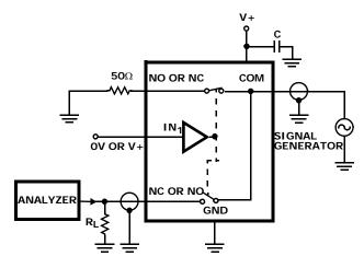
FIGURE 6. CROSSTALK TEST CIRCUIT
