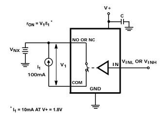
FIGURE 5. ron TEST CIRCUIT
