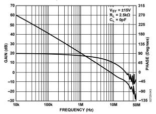
Figure 48. Frequency Response of the AD8510/AD8512/AD8513
