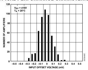
Figure 7. Input Offset Voltage Distribution
