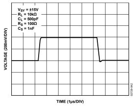
Figure 47. Capacitive Load with Snubber Network
