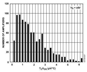
Figure 37. AD8513 T<sub>C</sub>V<sub>OS</sub> Distribution
