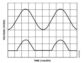
Figure 51. Half-Wave Rectifier Signal (OUT A in Figure 50)
