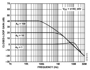
Figure 19. Closed-Loop Gain vs. Frequency
