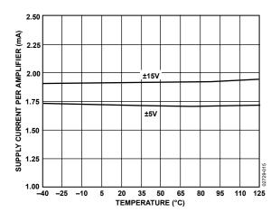
Figure 15. AD8512 Supply Current per Amplifier vs. Temperature
