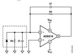
Figure 53. Equivalent Preamplifier Photodiode Circuit
