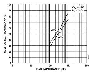
Figure 35. Small-Signal Overshoot vs. Load Capacitance
