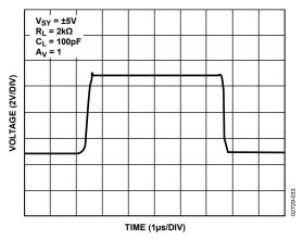
Figure 33. Large-Signal Transient Response
