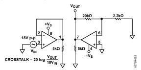
Figure 56. Crosstalk Test Circuit
