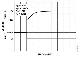
Figure 43. Positive Overload Recovery
