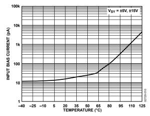
Figure 10. Input Bias Current vs. Temperature
