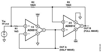
Figure 50. Half-Wave and Full-Wave Rectifiers
