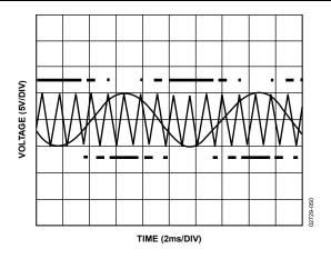
Figure 55. Pulse-Width Modulation
