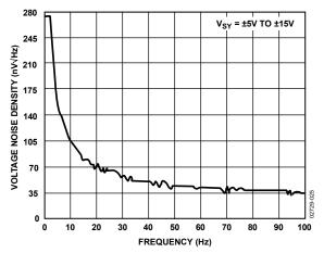
Figure 25. Voltage Noise Density vs. Frequency
