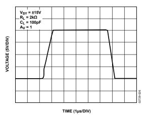
Figure 26. Large-Signal Transient Response
