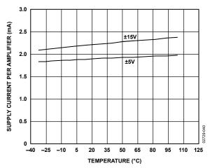
Figure 40. AD8513 Supply Current per Amplifier vs. Temperature
