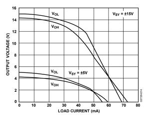
Figure 14. AD8510/AD8512 Output Voltage vs. Load Current
