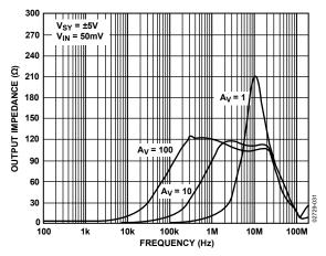
Figure 31. Output Impedance vs. Frequency
