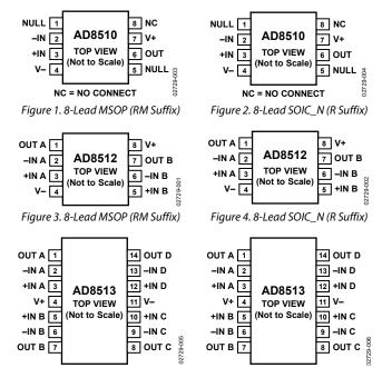
Figure 5. 14-Lead SOIC\_N (R Suffix)
