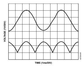
Figure 52. Full-Wave Rectifier Signal (OUT B in Figure 50)
