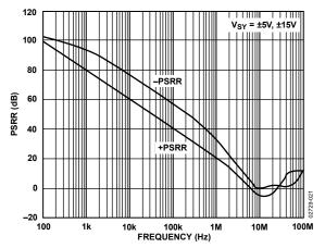
Figure 21. PSRR vs. Frequency
