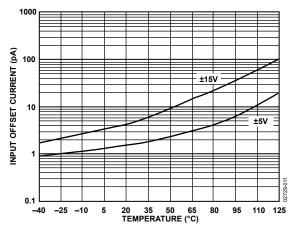
Figure 11. Input Offset Current vs. Temperature
