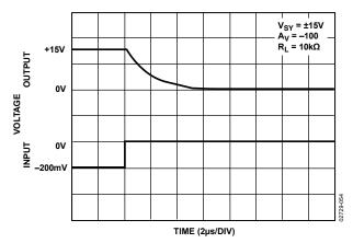
Figure 44. Negative Overload Recovery
