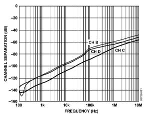
Figure 57. Channel Separation
