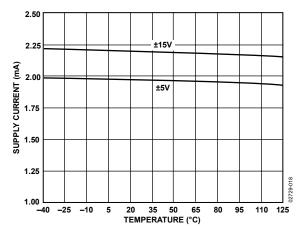
Figure 18. AD8510 Supply Current vs. Temperature
