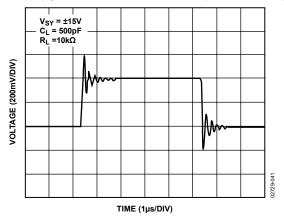
Figure 46. Capacitive Load Drive Without Snubber
