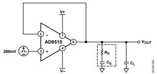
Figure 45. Snubber Network Configuration
