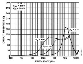
Figure 22. Output Impedance vs. Frequency
