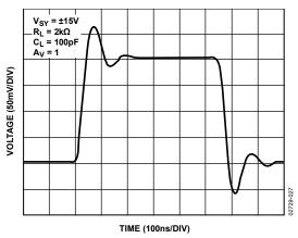
Figure 27. Small-Signal Transient Response
