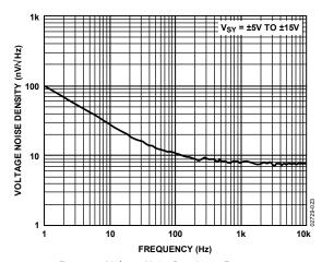
Figure 23. Voltage Noise Density vs. Frequency
