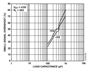
Figure 28. Small-Signal Overshoot vs. Load Capacitance
