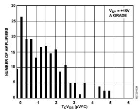
Figure 9. AD8510/AD8512 T<sub>C</sub>V<sub>OS</sub> Distribution
