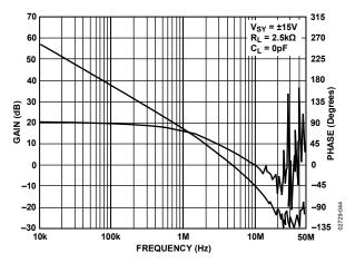
Figure 49. Frequency Response of Competitor A
