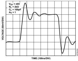
Figure 34. Small-Signal Transient Response
