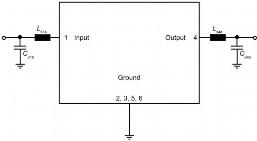
Figure 3: Schematic of matching circuit.
