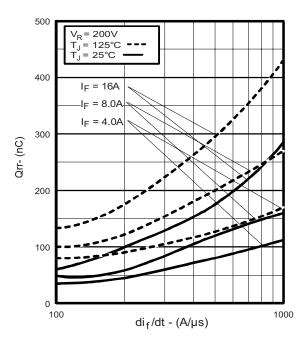
Fig. 7 - Typical Stored Charge vs. dl<sub>F</sub>/dt (Per Leg)
