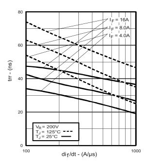
Fig. 5 - Typical Reverse Recovery Time vs. dl<sub>F</sub>/dt (Per Leg)
