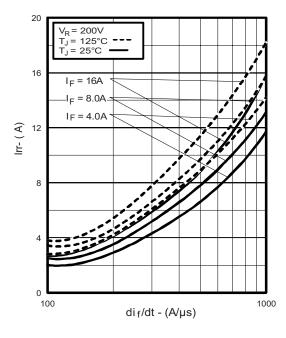
Fig. 6 - Typical Recovery Current vs. dl<sub>F</sub>/dt (Per Leg)
