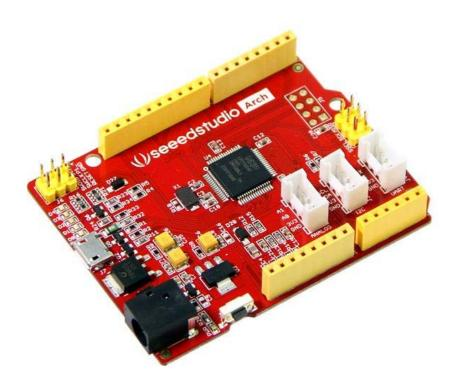
Arch V1.1 is an mbed enabled development board with Arduino form factor and Grove connectors for rapid prototyping. With a variety of Shield and Grove modules, mbed SDK and lots of software libraries, you can rapidly build a prototype.
