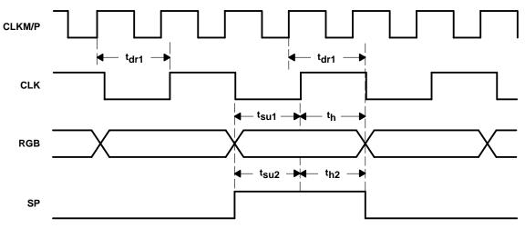
Figure 1. Output Setup and Hold Time
