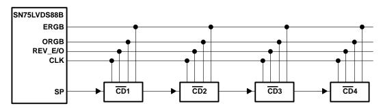
Figure 4. Application Block Diagram
