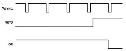
Figure 3. Reset Waveform
