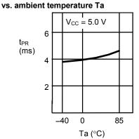
2. 5 Write time t<sub>PR</sub> vs. ambient temperature Ta
