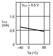
1.9 Current consumption (WRITE) I<sub>CC2</sub> vs. ambient temperature Ta
