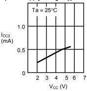
1. 12 Current consumption in standby mode  $I_{\rm SB}$  vs. power supply voltage  $V_{\rm CC}$
