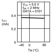
1.3 Current consumption (READ) I<sub>CC1</sub> vs. ambient temperature Ta
