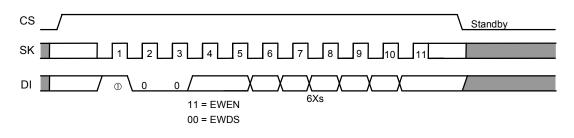
Figure 19 Write Enable / Disable Timing (S-93C56B, S-93C66B)
