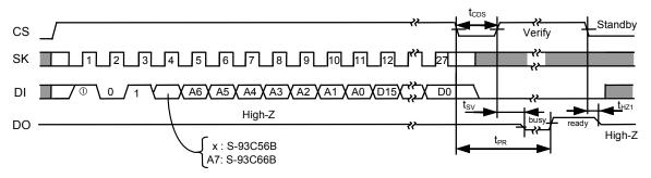
Figure 11 Data Write Timing (S-93C56B, S-93C66B)
