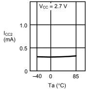
1. 11 Current consumption in standby mode I<sub>SB</sub> vs. ambient temperature Ta
