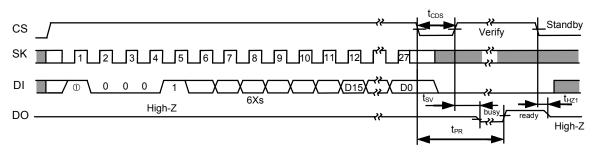
Figure 15 Chip Write Timing (S-93C56B, S-93C66B)
