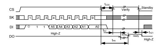
Figure 12 Data Erase Timing (S-93C46B)
