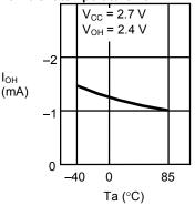
1. 25 High-level output current I<sub>OH</sub> vs. ambient temperature Ta
