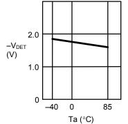
1. 32 Low supply voltage release voltage +V<sub>DET</sub> vs. ambient temperature Ta
