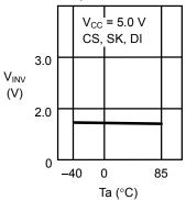
1. 31 Low supply voltage detection voltage -V<sub>DET</sub> vs. ambient temperature Ta
