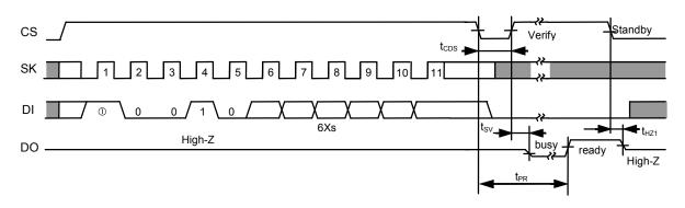
Figure 17 Chip Erase Timing (S-93C56B, S-93C66B)
