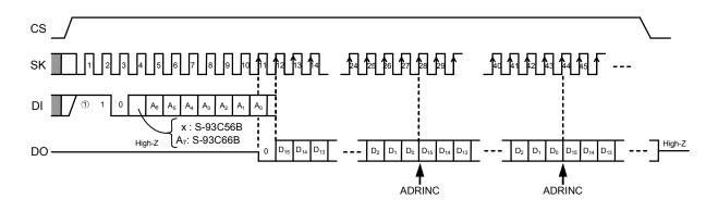
Figure 9 Read Timing (S-93C56B, S-93C66B)
