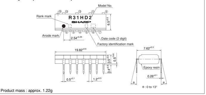
(Note) To radiate the heat, solder the lead pins ④ to ⑦, ⑨ on the pattern of the PCB without using a socket such that there is no open pin left.
