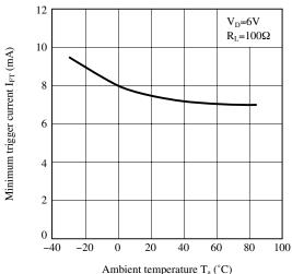
Fig.6 Holding Current vs.
