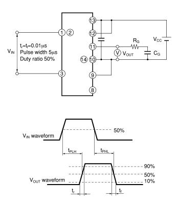
Fig.9 Test Circuit for Overcurrent Detection Voltage, Overcurrent Detection Voltage Hysteresis
