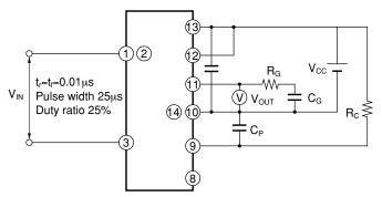
Fig.14 Error Signal "High→Low" propagation Delay Time, Error Signal Output Pulse Width
