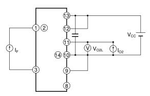
Fig.2 Test Circuit for O<sub>2</sub> High Level Output Voltage
