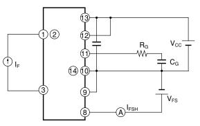
Fig.13 Test Circuit for O<sub>2</sub> "High→Low" Propagation Delay Time at Overcurrent Protection, O<sub>2</sub> Fall Time at Overcurrent Protection
