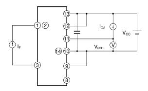
Fig.4 Test Circuit for O1 Leak Current
