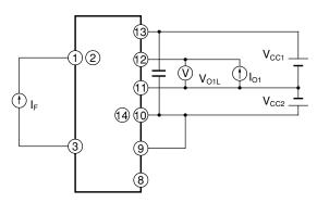
Fig.3 Test Circuit for O<sub>2</sub> Low Level Output Voltage
