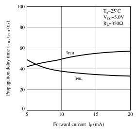
Fig.12 Propagation Delay Time vs.
