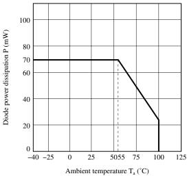
Fig.4 Total Power Dissipation vs. Ambient Temperature
