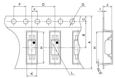
**Dimensions List** (Unit: mm) C Е F D G A 12.0±0.3  $5.5^{\pm0.1}$  $1.75^{\pm0.1}$  $8.0^{\pm0.1}$  $2.0^{\pm0.1}$  $4.0^{\pm0.1}$  $\phi 1.5^{+0.1}_{-0}$ Н K L Ι J  $7.5^{\pm0.1}$  $0.3^{\pm0.05}$ 2.3<sup>±0.1</sup> 3.1<sup>±0.1</sup> φ1.6<sup>+0.1</sup>
