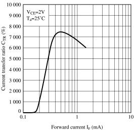
Fig.9 Collector Current vs. Forward Current
