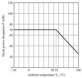
Fig.4 Total Power Dissipation vs. Ambient Temperature
