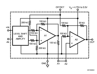
FIGURE 8. Mid-Rail Adjustment Pin Schematic
