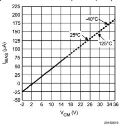
Input Bias Current Over Temperature (A2 Inputs)
