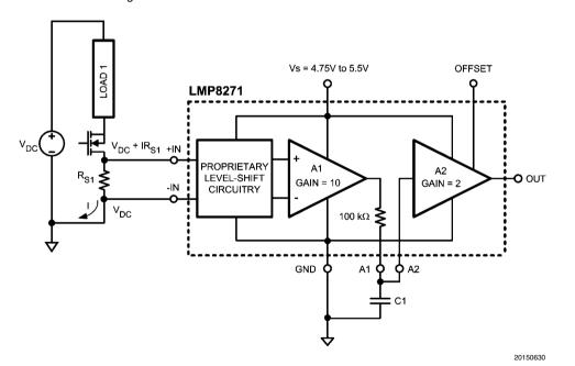
FIGURE 11. Low Side Current Sensing
