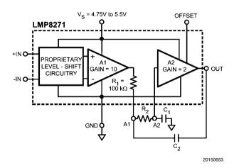
FIGURE 6. Low-Pass Filter With LMP8271
