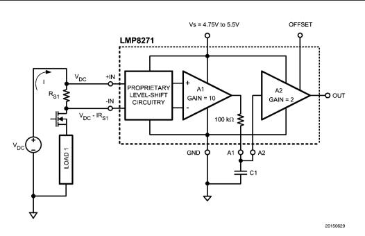
FIGURE 10. High Side Current Sensing
