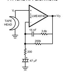
$A_V = 34.5$  F = 1 kHz  $E_n = 0.38 \text{ }\mu\text{V}$  A Weighted
