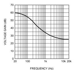
Figure 28. NAB Preamp Voltage Gain vs Frequency  $V_{\text{IN}}$  = 10mV,  $A_{\text{V}}$  = 34.5dB, f = 1kHz
