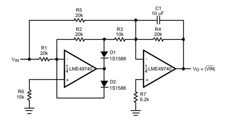
Figure 35. AC/DC Converter
