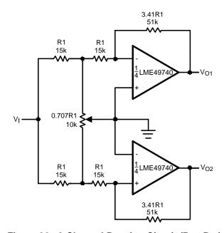
Figure 36. 2-Channel Panning Circuit (Pan Pot)
