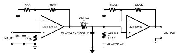
Note: 1% metal film resistors, 5% polypropylene capacitors
