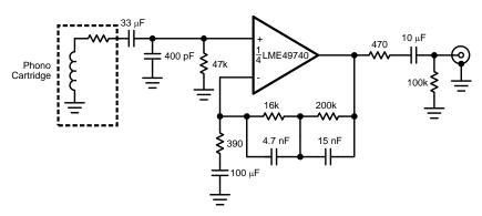
$\begin{array}{l} A_v = 35 \text{ dB} \\ E_n = 0.33 \text{ } \mu\text{V} \\ \text{S/N} = 90 \text{ dB} \\ \text{f} = 1 \text{ kHz} \\ \text{A Weighted}, \text{ V}_{\text{IN}} = 10 \text{ mV} \\ \text{@f} = 1 \text{ kHz} \end{array}$
