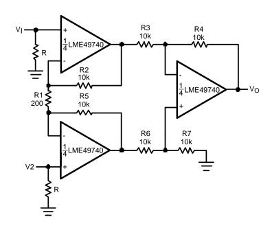
If R2 = R5, R3 = R6, R4 = R7  $v_0 = \left(1 + \frac{2R2}{R1}\right) \frac{R4}{R3} (v_2 - v_1)$  Illustration is:  $v_0 = 101 (v_2 - v_1)$
