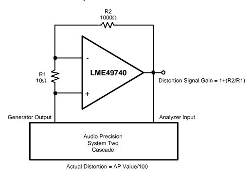
Figure 23. THD+N and IMD Distortion Test Circuit
