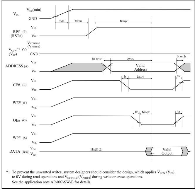
Figure A-1. AC Timing at Device Power-Up
