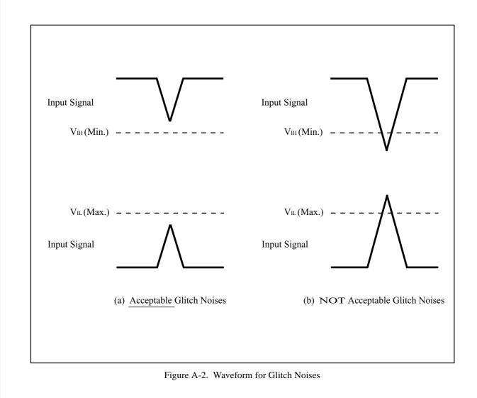
See the "DC CHARACTERISTICS" described in specifications for  $V_{IH}$  (Min.) and  $V_{IL}$  (Max.).
