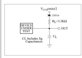
Figure 5. Transient Equivalent Testing Load Circuit
