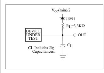
Figure 5. Transient Equivalent Testing Load Circuit
